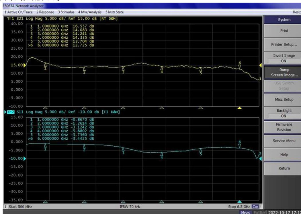
15W, 1-6GHz, 28V GaN 射频功率晶体管
